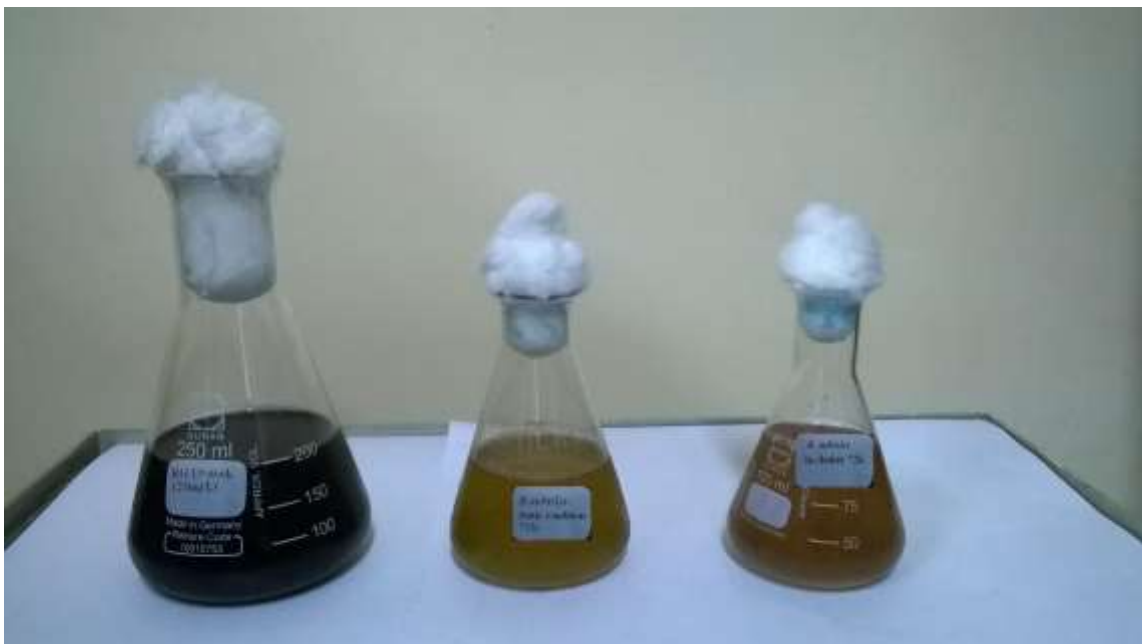
Figure 2: Experimental observation of the decolorization of RG 19 using B. subtilis after 72h of incubation period
